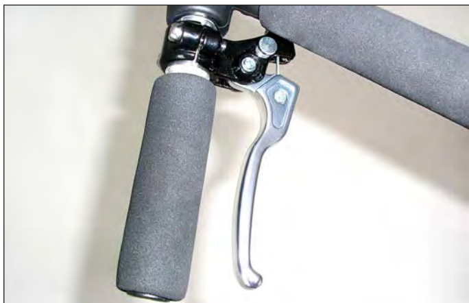
Brake lever in the parked position
